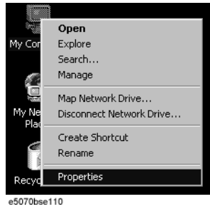
Figure 4-17 Opening System Property Window
